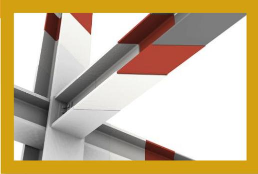
Thin film intumescent coating designed for the fire protection of steelwork for up to a 3 hour fire rating, depending on the steel design. Intumescent fireproofing is a spray applied coating that swells or intumesces to many times its original wet film thickness as a result of heat exposure. As the product expands, it insulates and protects structural steel members from the heat of a fire.
